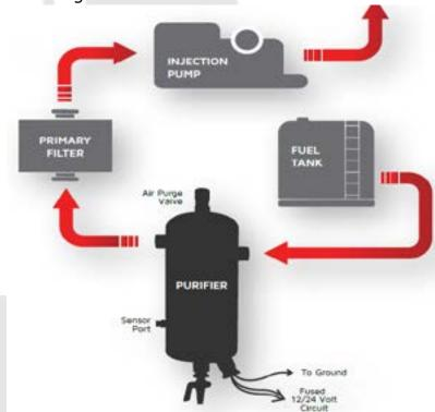
The Fuel Purifier removes up to 99.8% of free water and up to 95% of other heavy contaminants before it ever reaches your engine's primary filter.
