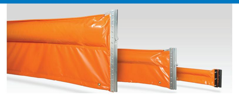
Floating containment boom is manufactured from a variety of extremely durable, flexible thermoplastic fabrics. These fabrics are dielectrically sealed to form enclosures for flotation logs and for the galvanized chain ballast that also serves as a tension member. A skirt that extends below the surface of the water provides a flexible floating barrier.
