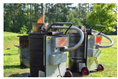
The Drug Terminator uses what is specified by ISO Standards as a removable head or "open-end" drum. The measurement of this drum type is standard around the world. ISO 15750, published in 2002, traditionally identifies this drum as being 55 American Gallon. Drug Terminator, Mobile Incinerator for Disposal of Illicit DrugsUS Norm ANSI/ASC MH2-1985  $\cdot$  22 1/2 in  $\pm$  1/16 I.D. European Standard EN 209  $\cdot$  571.5mm +1/-0.5 I.D.
