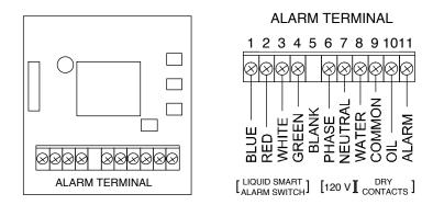
\* All components are pre-wired for plug and play installation. To access alarm circuit board and dry contacts for remote monitoring, remove back panel. The dry contacts are rated for 60V AC or DC, 1 amp maximum.
