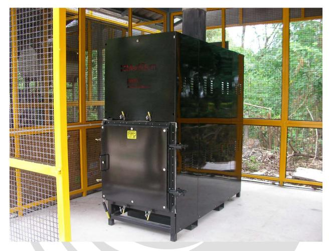
ProBURN is a diesel-fueled medical waste incinerator for hospitals and clinics. It is environmentally safe, compact, portable, and easy to operate.
